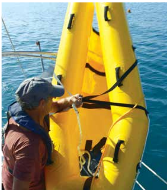
Crew can lift the Sea Rescue Sled horizontally using a winch or block and tackle.
