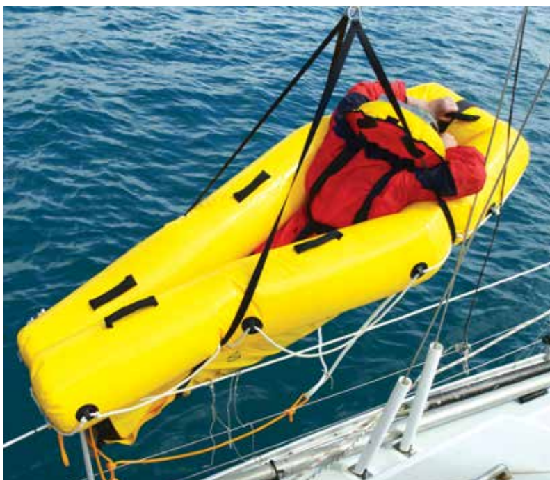
Crew can lift the Sea Rescue Sled horizontally using a winch or block and tackle.
